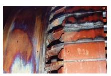
Rotor core damage due to broken bars
